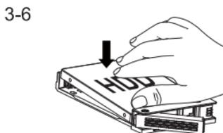
Note: Firmly press down the backside of the drive to secure the drive onto the tray.
