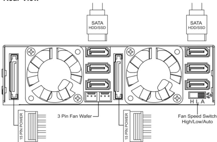
Note: In order to function properly, please connect both 15 pin power connectors to the enclosure when using the device.
