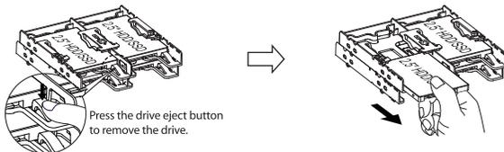
Press the drive eject button to remove the drive.
